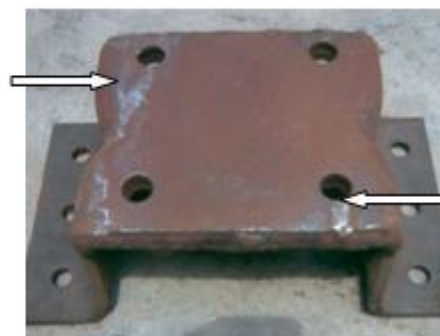
Fig. 1.5 Failure points in the bracket
